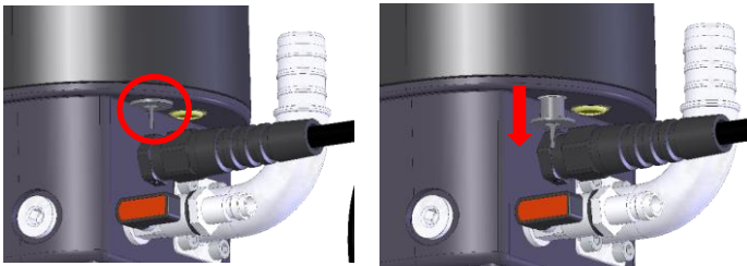
Fig. 3: Pressure relief valve with protective cap
